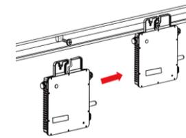
\*Note: Please install the microinverter at least 50cm above the ground/roof for better communication with Hoymiles DTU.
