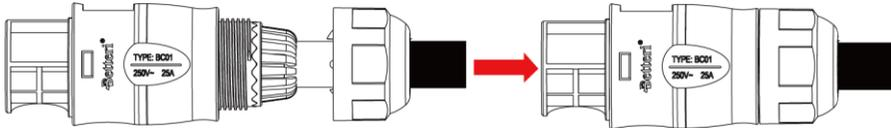
B) Connect the AC end cable to the AC male connector of the first microinverter to complete the circuit.
