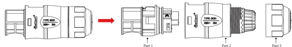
2. Insert the AC cable from Part 3 to Part 2, and complete the wiring for the L, N and Ground inside Part 1 AC port accordingly:
